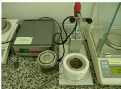
Determining humidity level with non-destructive method, fot. Dagmara Topola
